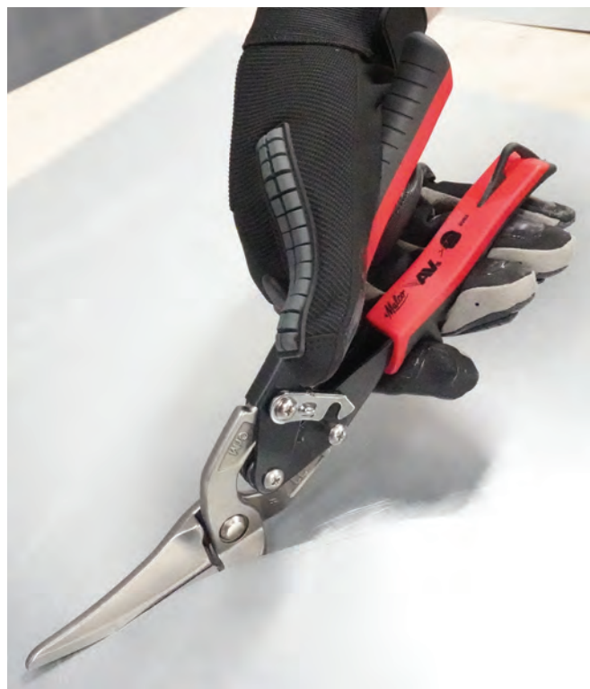
This pair of offset aviation snips made by Malco Tools has handles that are angled up from the cutting surface, allowing more hand clearance and control for more accurate, precise cuts with less hand strain.
