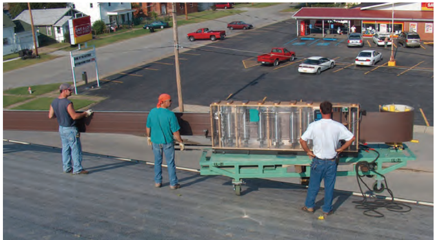
Berridge Manufacturing's CL 21 portable roll former produces a 1-1/2-inch cee-lock snap lock panel. BERRIDGE MANUFACTURING PHOTO
