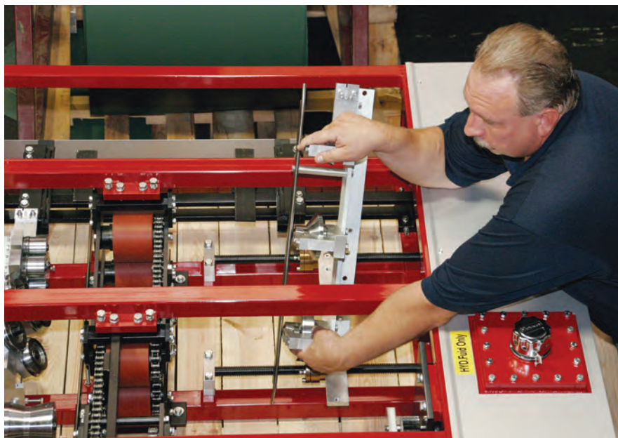
Mike Gorski, senior roll former technician at Englert inserts tooling into a Metal Man machine.
