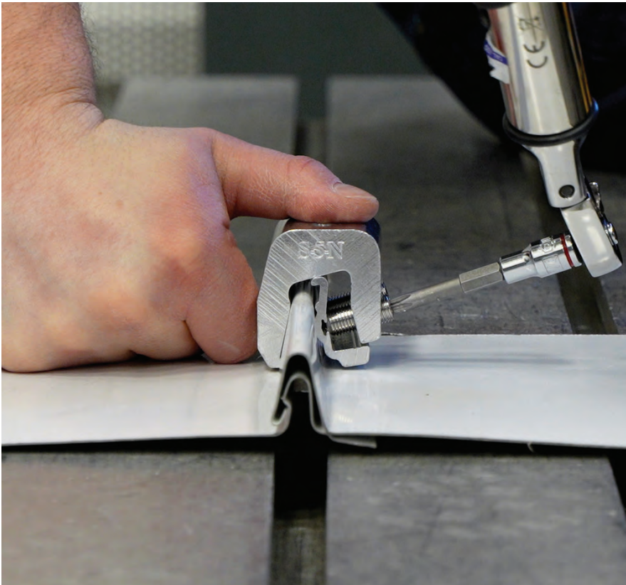
Non-penetrating clamps will dimple the seam material, forming a mechanical interlock between the clamp, seam and setscrew when tightened. PHOTO COURTESY OF S-5!
