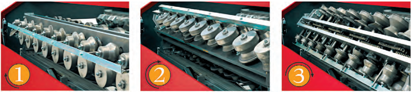
Cassettes for MetalForming's Quadro roll former (bottom) and a sequence of photos (top) illustrating a changeover. METALFORMING PHOTO
