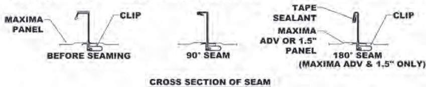
Mechanical seam inspection (Maxima Panel). COURTESY OF MCELROY METAL.
