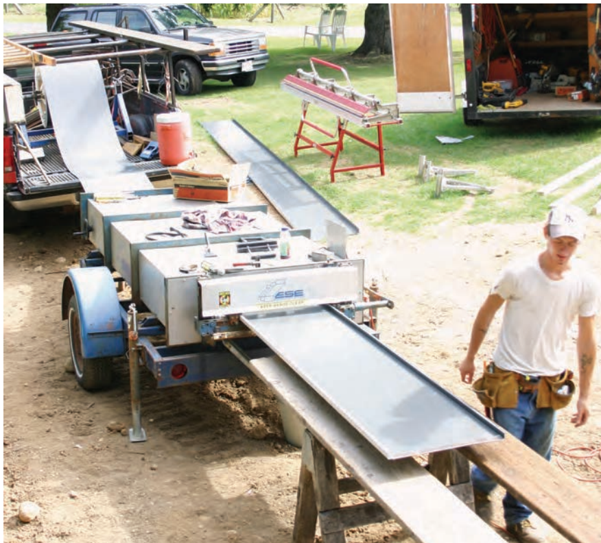
Jason Golke pulls the handle to activate the guillotine on the roll former that cuts the panels to an exact length.
