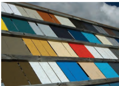
Sherwin-Williams tests for weatherability. PHOTO COURTESY OF SHERWIN-WILLIAMS COIL COATINGS
