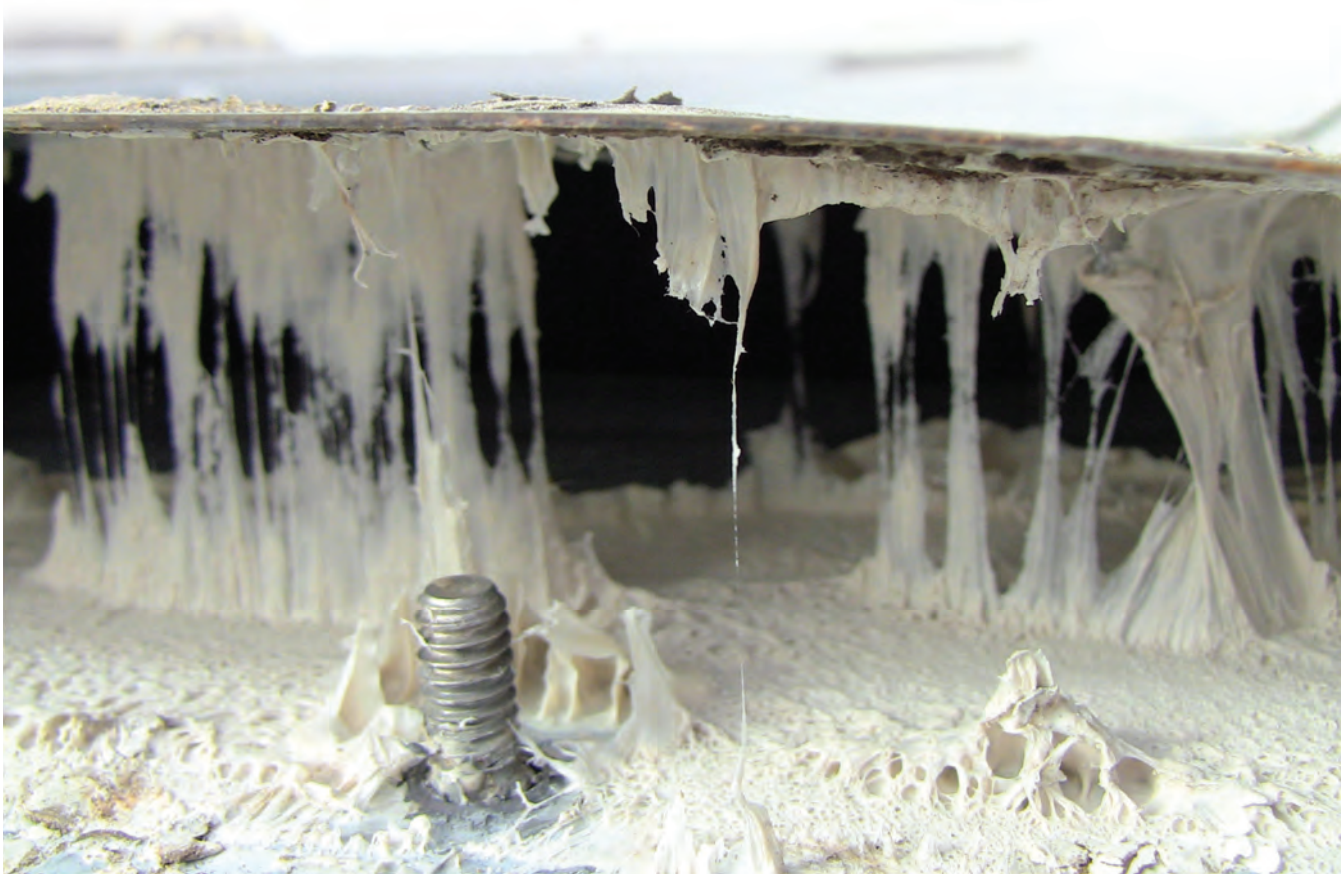
Figure 1: Webbing, elasticity and adhesion of a proven butyl formulation within a joint after 33.5 years of service. PHOTO COURTESY OF ROB HADDOCK, METAL ROOF ADVISORY GROUP LTD.
