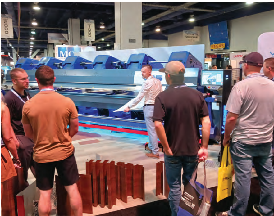
ASCO USA held equipment demonstrations over the course of the three-day trade show. Demonstrated here is the V2.5 long folder.
