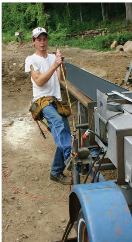
Jason Golke pulls the handle to activate the guillotine on the roll former that cuts the panels to an exact length.
