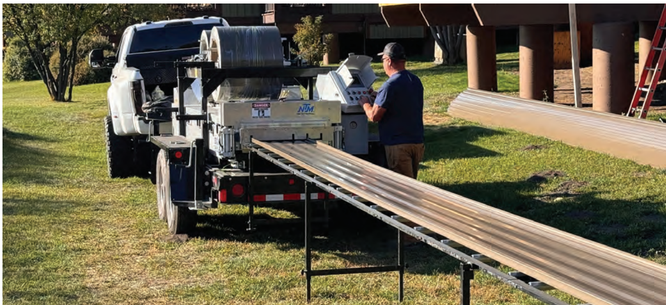
Benefits of roll forming onsite include reduced waste, faster panel production, and minimal downtime. Only you can determine if the investment in a portable roll former is right for your business. PHOTO COURTESY OF NEW TECH MACHINERY
