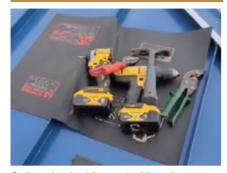
Safety Assist Magnetic Mats for working on steel roofing. Standing Seam mats, 21"x28". Diamond deck rubber grip surface integrated to heavy canvas backer, two 10"x21" super strong flexible magnets. Nonslip rubber coating over magnetic underside. 8" fabric center lays over ribs. Helps keep tools and workers in place.
