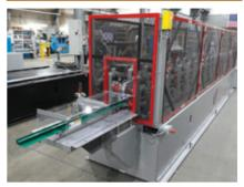
The F&J Single Trim Rollformer features cast roll-forming stands and bearings blocks, safety swing guarding and in house designed roller die tooling. The drive system can be electric, hydraulic or mechanical.
