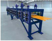
Our customer-inspired Soffit Line uses standard 20.125" coil stock to optimize inventory and cut costs. Features include concealed "S lock" lap, standard rib height, flat top rib for easy fastening, unique nail slots and weep holes for horizontal installs, and speeds over 150 feet per minute for increased productivity.
