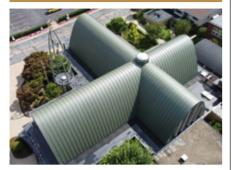
The Batten-Tite<sup>™</sup> architectural metal roof panel system is designed for roofing applications with slopes of 3" per foot or greater, as well as vertical wall applications. With 1-7/8" battenstyle ribs and custom panel widths up to 44-1/2" (nominal coverage), Batten-Tite is perfect for domes, concave and convex curves, and conical tapers. Available in continuous lengths up to 45'.
