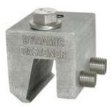
Dynamic Fastener's new DC-NFTG DYNA-CLAMPS® are non-ferrous, non-piercing clamps for attachment to standing seam metal roofs. They're made from aircraft-grade 6005A T61 aluminum de-signed for use with nail flange standing seam roof profiles. The clamps are prepackaged with all necessary mounting hardware, both the non-piercing setscrews and stainless steel bolts.
