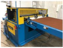
The Bradbury B.O.S.S.<sup>™</sup> shear provides high production rates with close tolerance shearing. The shear can be equipped with notching or slitting – allowing the B.O.S.S.<sup>™</sup> to be used for various applications. The intelligent drive and shear system allows the B.O.S.S.<sup>™</sup> to be closecoupled to a new or existing roll former.
