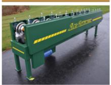
Acu-Form Trim Roll Formers are built with longevity and ease of operation in mind , while producing precise parts in a variety of profiles, including custom matches. Saving you time which is money. All our forming dies are made from D2 tool steel for a longer wear life. These machines can be powered by Electric, Hydraulic or Mechanical.
