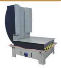
Coil Up Enders are available from Stoll Metal Works. Your choice of power source; there are three options available: electric, hydraulic, or engine driven. Our Up Enders are rated for 10,000 lb. coils. The Electric model is available with an optional wireless remote.
