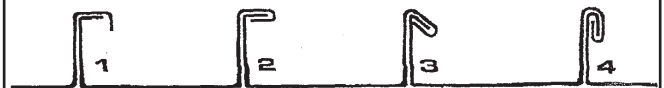
Before using this tool prepare seam up to position 2 with above single lock hand tool.
