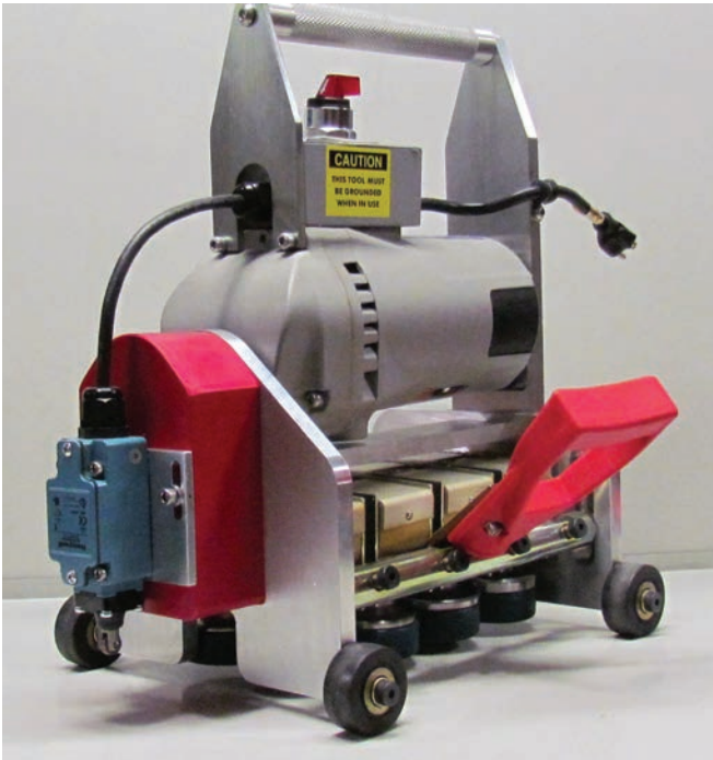
When the runner switch at the front of this seaming machine extends, it cuts power to the wheels, ensuring the seamer doesn't run off the roof. PHOTO COURTESY OF ROLLFORMER LLC
