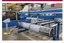
ASC's custom-designed rollup stations allow manufacturing residential and commercial roll-up doors widths between 3.5 ft and 20 ft. Optional curtain assembly tables allow the easy pre-assembly of the door panels before the seaming process. Infeed/assembly tables feature an automated tensioning device to adjust the tension when winding seamed panels onto the drum.
