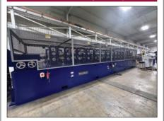
Bradbury Rollforming Line to produce interlocking wall panels features a coil car, 20,000 lb stock reel, roller straightener, and a hydraulic punch/notch/cutoff system before material enters the 16-pass rollformer. With Bardie Cartridge technology for automatic gauge adjustment, D-2 roll tooling, and a servo-driven Anti Flare Fixture, precision and efficiency are ensured throughout the process.
