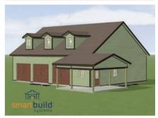
SmartBuild is a web-based design software built specifically for post-frame construction. Building geometry is defined using a 3D user interface. The software automatically generates material lists and pricing. Features include interior floor plans for barndominium designs, lofts, mezzanines, dormers, windows, doors, and multiple material types for framing, sheathing, and trim.
