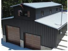
True Board and Batten Steel Siding offers the beautiful look of realistic vertical wood siding, without preventative maintenance. This 26ga, 10" coverage, 3/4" batten steel siding features crinkle textured paint or wood-grain prints on a concealed-fastened panel. It's not susceptible to termite damage, chipping, cracking, or splitting, doesn't need repainting, and is extremely energy efficient.
