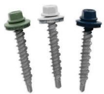
The "PG" woodscrew fastener attaches metal panels to wood-frame applications. It's available in 20 colors and features a #11 Hi-Lo Thread, resulting in better strip to set ratio. The 1/4" hex washer head reduces the screw appearance, and the EPDM bonded 5mm galvanized washer creates a superior seal.
