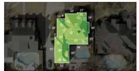
Roof data from EagleView report. PHOTO COURTESY OF EAGLEVIEW
