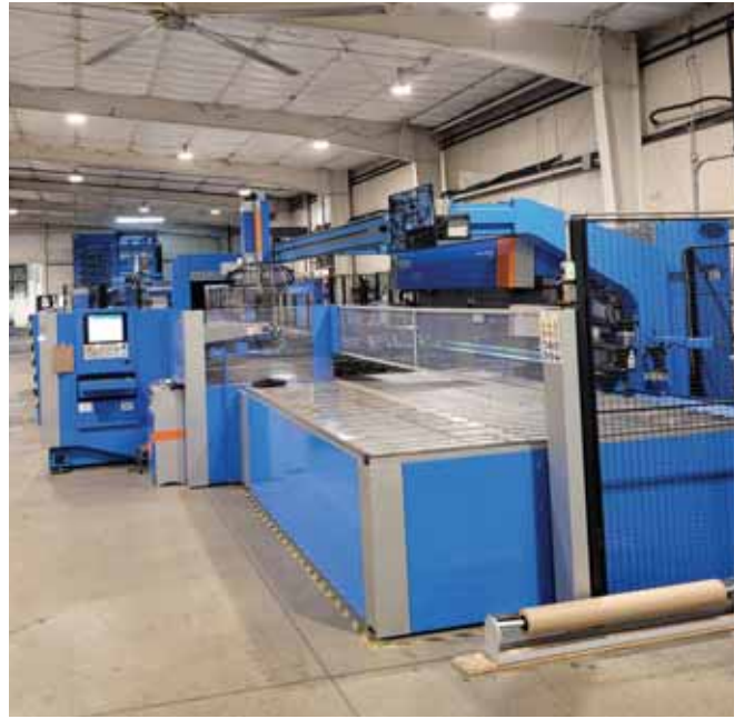
An Automated Self loading Multi Stage Line Capable of Punching, shearing, tapping, sorting, bending. PHOTO COURTESY OF RAYTEC
