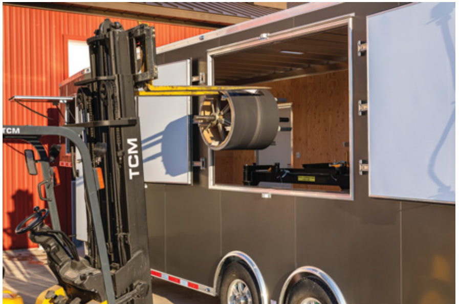
Side doors are convenient for loading and unloading coil. PHOTO COURTESY OF FORMWRIGHT (FORMERLY MASTERPIECE METAL ROOFING)
