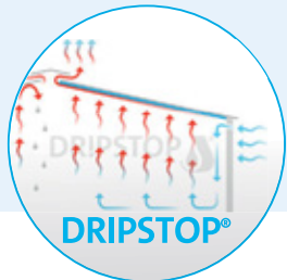
Effective condensation control requires good building ventilation
