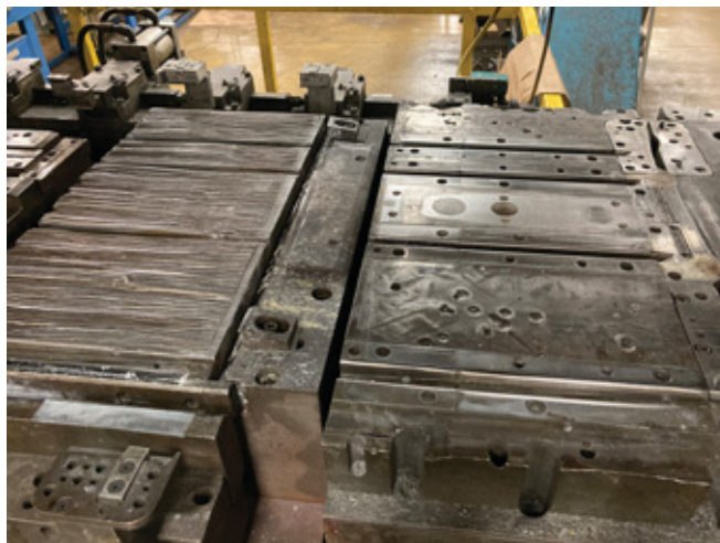
An up-close look at the design plates the coil is sent through during the stamping process.
