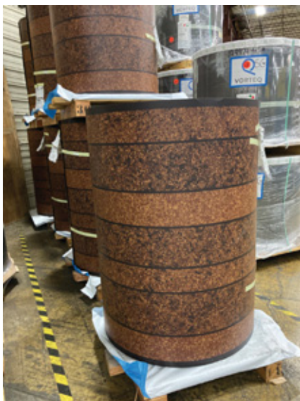
Coil arrives pre-painted, sometime with a special effect as shown on the left, through the stamping press to create the final 3-D shingle. Photos by Sharon Thatcher
