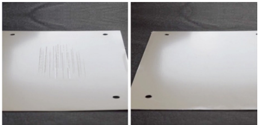
Testing results demonstrate the abrasion protection offered by Steel Shield. On the left: an unprotected steel plate. Above right, the plate has been protected with SteelShield.
