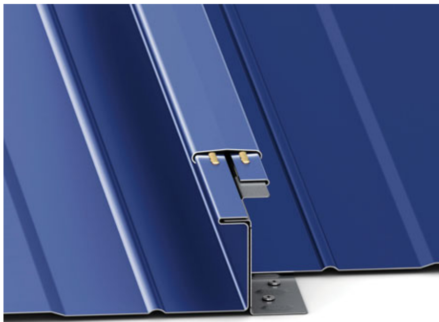
Since symmetrical panels float on a fixed clip, the panel length is not limited by the clip.
