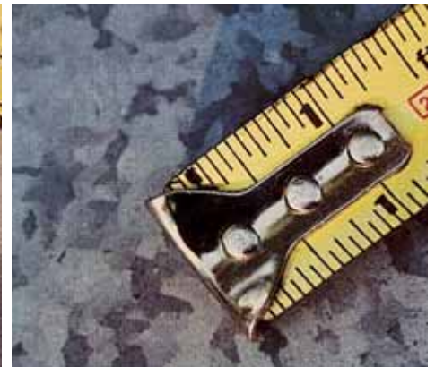
Differing spangles of Galvalume (left) and galvanized (right). PHOTOS BY DEREK A. HODGIN.
