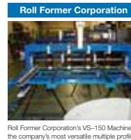
Roll Former Corporation's VS-150 Machine is the company's most versatile multiple profile machine forming 1" & 1½" standing seam profiles—complete with hydraulic drive and shear as well as adjustable panel width of 9" to 24". The VS-150 is offered with Optional Panel Dies giving the contractor up to eight (8) different panel profiles. Snap Lock & Tong Board & Batter Panel and Cap profiles. All of this with quick and easy changeover! Call us today at 215-937-2511.
