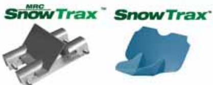
ST Fastening Systems offers Snow Trax snow-retention guards for exposed fastener roofs, and the MRC Snow Trax roof clamp for standing seam roofs. The Snow Trax is 16 gauge 304 stainless steel available in more than 20 powder coated colors. Its adhered rubber gasket eliminates the need for additional sealant. The MRC is extruded aluminum and a colored rail slices through the clamp grooves to provide maximum protection from snow and ice.
