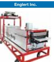
The Englert Metal Man FP1300 Panel Rollformer is a state-of-the-art roll forming machine that runs the A1300 Panel in various gauges and types of materials with near infinite options for scrap. On-site fabrication eliminates shipping costs and short shipments while reducing sizing errors and providing packaging and freight savings. Available in 16-inch and 20-inch coverage. Financing available.
