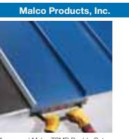
A compact Malco TSM Double-Cut TurboShear clearly navigates 90° outside angled standing seam panels. It can be paired with a Model DEFT 24-inch or DEFT 18-inch Folding Tool and SG11 Seamer with Vinyl Gripped Jaws, this trio is a complete system for making perfect drip edges in standing seam panels. Add a hand-operated ER3 Edge Roller to make precise trim-edge bends in standing seam and you have an arsenal of labor-saving Malco options from which to choose.
