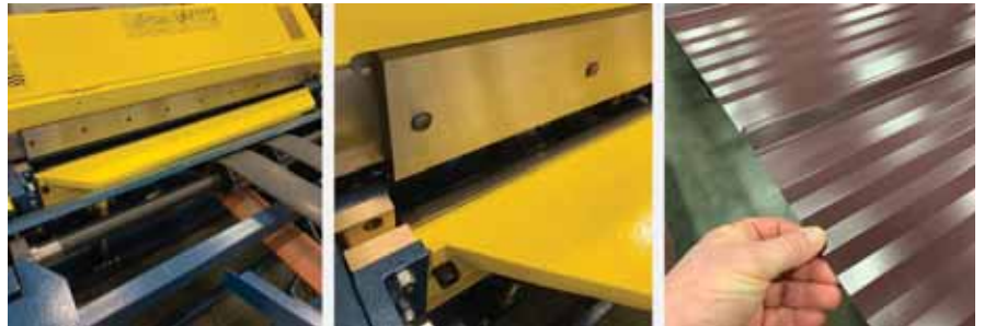
Monthly maintenance should include checking shear blades for wear and proper adjustment. Photo provided by Metal Rollforming Systems
