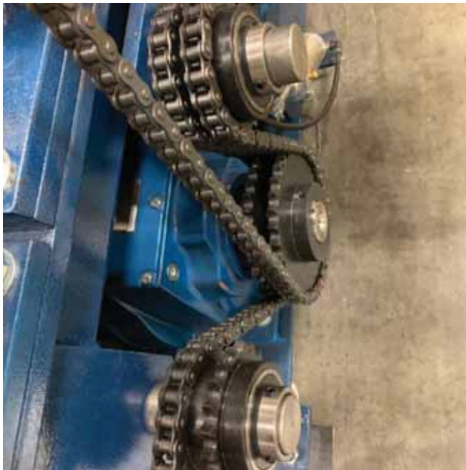
Part of weekly maintenance includes inspecting chain tension and lubricating with recommended lubricant. It’s clear why the chain on the left is going to provide more optimum performance than the one on the right. Don’t forget to use safety equipment when working with chains, however. Many accidents occur in this area of the machine. Photos provided by Metal Rollforming Systems
